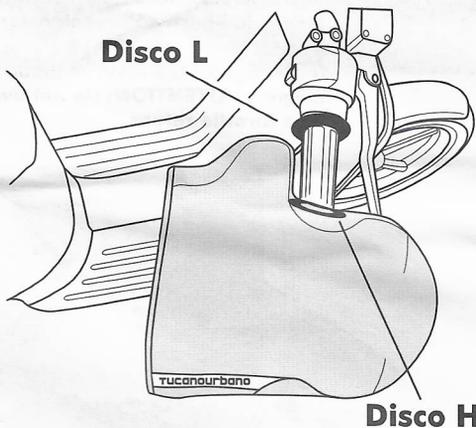
**GB** Slide **Disc L** onto the throttle grip as shown in the diagram. Slide the handlebar muff onto the scooter/motorbike's handlebar controls. Check that **Disc L** and **Disc H** are securely fitted together, as shown in the figure. Slide the handlebar muff R362X onto the controls of the scooter/motorbike, and ensure it is in the proper direction. Insert the grip in the large opening and the break lever in the small opening.
